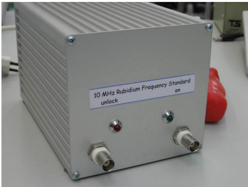
Fig.1: The closed aluminium cabinet with the Rubidium frequency standard LPRO-101 , a 24V switching power supply and a sine to TTL converter built in.
